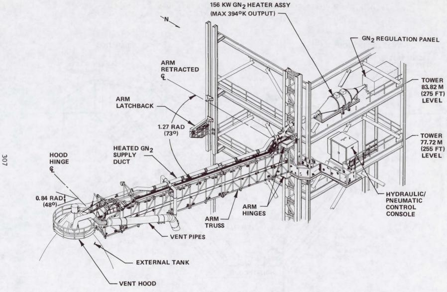
Figure 1. ET GOX Vent System Installation at Launch Complex 39A
