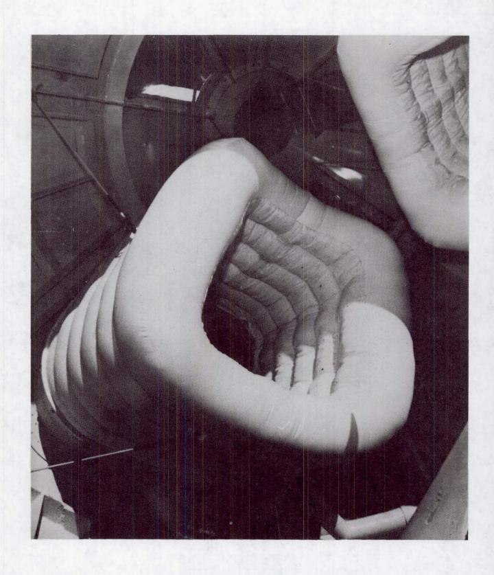
Figure 4. ET GOX Vent Inflatable Seals
